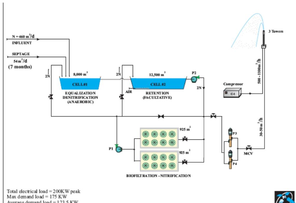
**Figure 3.5 Process Schematic – Warm Weather Operation**
